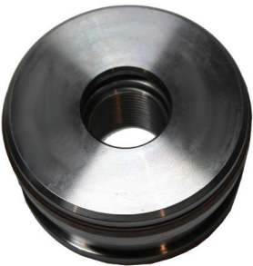
6. The PTFE seal is now assembled.
